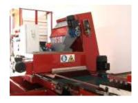
**Auto Soil filling:** This is an automatic mechanised system for soil filling in root trainer in desired quantity and the process is 10 time faster than manual soil filling.
